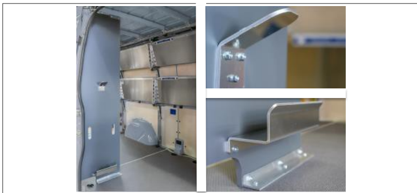
Figure 5: Hand truck mount without dolly (left), details (right)
