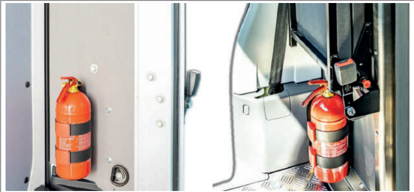
Figure 3: Fire extinguisher, on sliding cargo door (left), in driver's cab (right)
