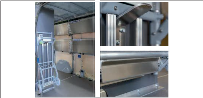
Figure 6: Hand truck mount with dolly (left), details (right)
