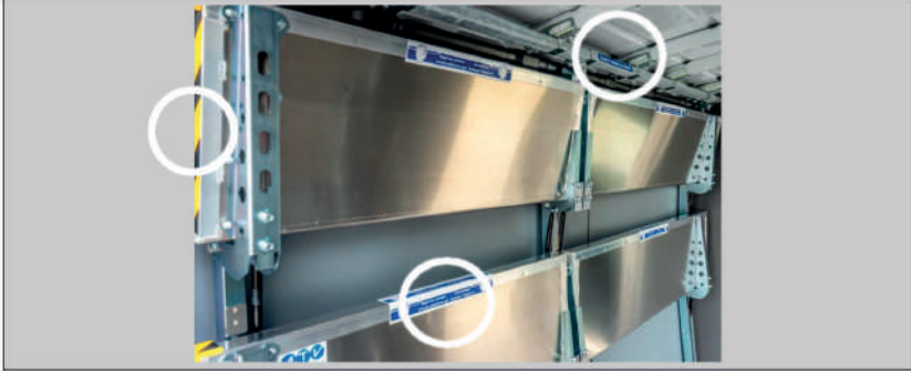
Figure 2: Shelving system detail, positions of warning signs
