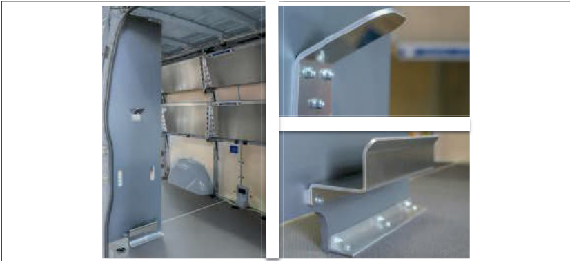
Figure 5: Hand truck mount without dolly (left), details (right)
