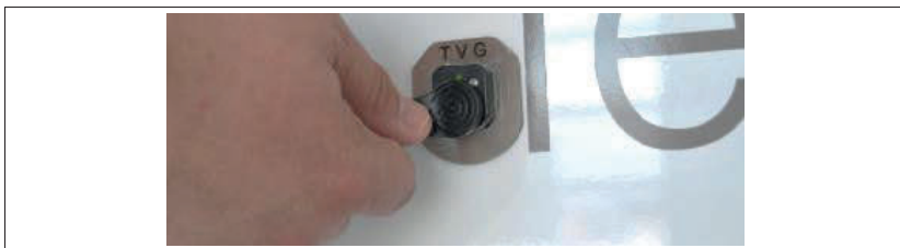
Figure 12: Locking system on cargo doors TVG brand, opening with Dalles key
