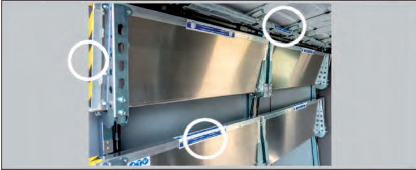
Figure 2: Shelving system detail, positions of warning signs
