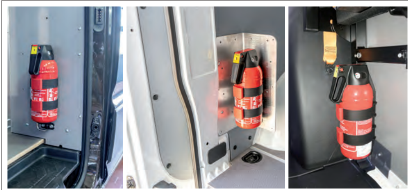
Figure 3: On the load compartment partition wall / behind sliding cargo door and in the drivers cab
