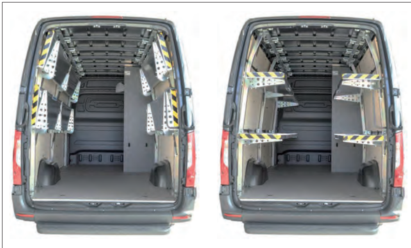
Figure 1: Shelving system raised (left), down (right)
