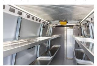
ATV partition wall with e-Slider (electric sliding door)
